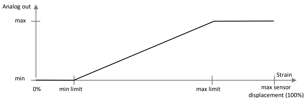
Figure 3: Analog output signal with taught limits.
