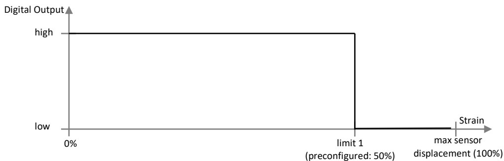
Figure 2: Digital output signal vs. displacement (with external pull-up resistor).
