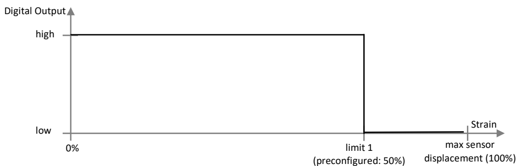
Figure 3: Digital output signal vs. displacement (with external pull-up resistor).
