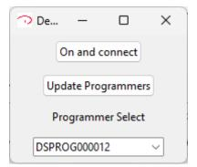
If the sensor was connected to the PC before starting the program, the programming adapter is already selected. Otherwise, connect the sensor, wait for 10 s for initialization by the operating system, press "Update Programmers" and select the proper adapter.
